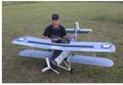
Paul McKeown's ESN Swordfish 88" has a Turnigy Motor 6364 and 10S batteries. It weighs 9.8kg
