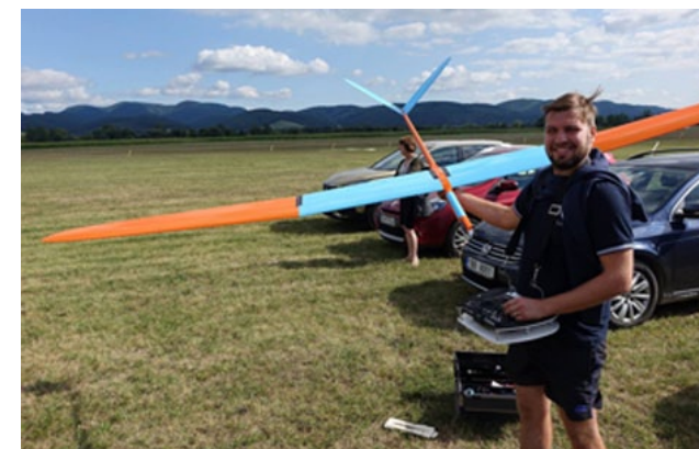
Interesting model seen in Slovakia - controls by wing twist with 9 servos in wing
