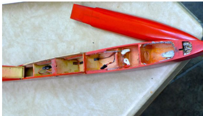
The original glider fuselage - note the huge lump of lead in the nose - now replaced with motor & LiPo.
