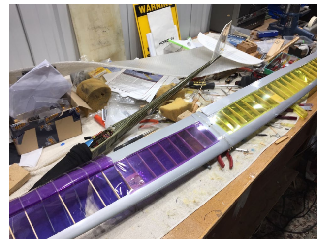
Byam Wight refurbished his Omega glider. Changed from 7-cell to 3S - blew the covering off the wing as he climbed!
