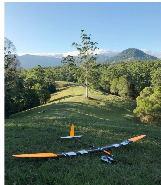
Right: New Viator F5j glider by Kane Morley of Tyalgum. Hails from Russia, is 3.2m wingspan and weighs about 1kg. Flies beautifully with a Mega 1615/5 CE inner-runner motor. The thin wing and low weight combine to make it a great thermal machine.
