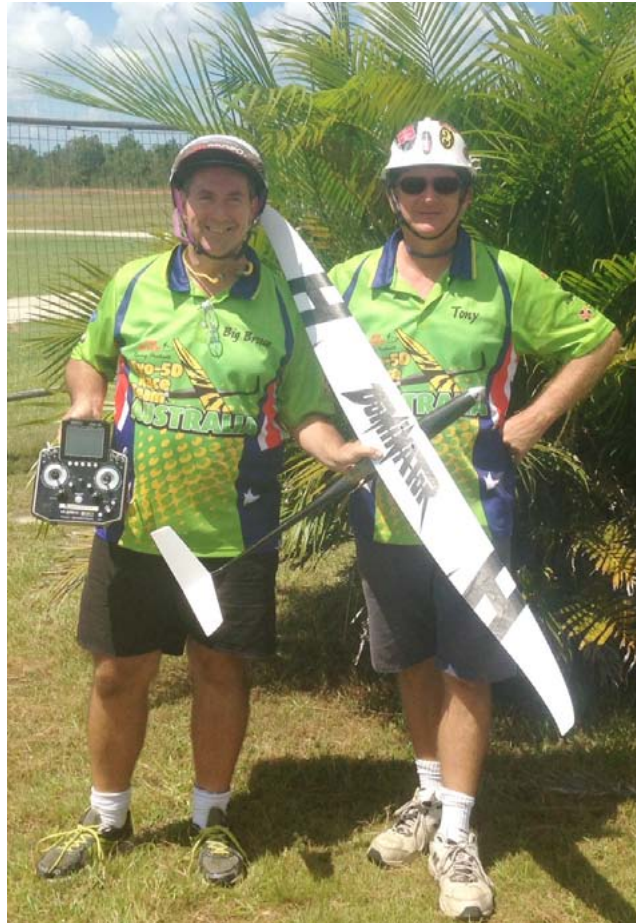
Bruce (left) and Tony (right) with the Dominator model produced by Bruce. 1.42m wingspan with a 7% thick wing - and weighs in at 1.0kg. Direct drive - Leomotion or Neu motors 2100 to 2300 Kv giving 32,000 rpm with 5.25 x 6.25" prop. Gear drive - Leomotion 4200 Kv with 6.7:1 gear and a 12x25 sawtooth prop running at 10,000 rpm. 1800-5S LiPo through a Jeti Mezon Lite 90 ESC - draws 60A in flight for a 58 second run time - at speeds up to 320 km/hr in straights, 270 km/hr in turns! Bruce has now produced over 60 of these models!
