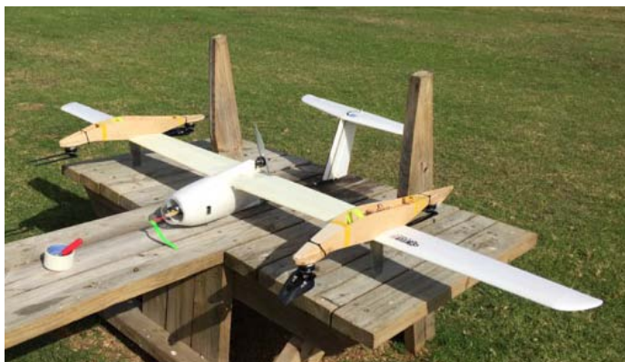
A drone being prepared for the Search & Rescue event at Kingaroy - an attempt at VTOL and transition to forward flight - check Youtube for more samples of people who have achieved this!
