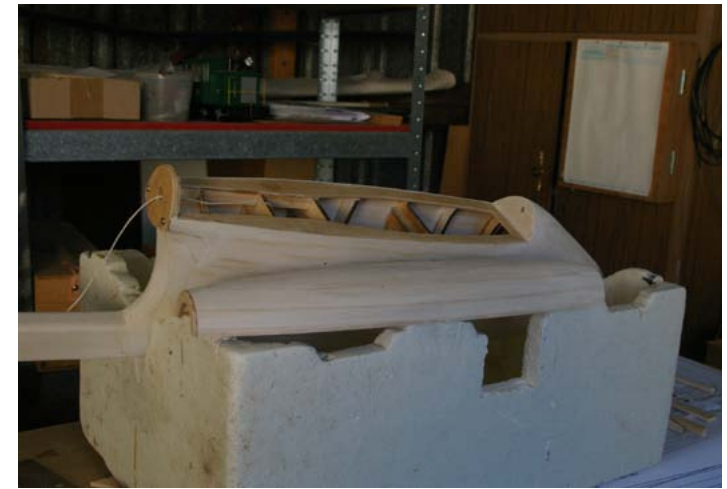
Nose planked with top hatch removed
