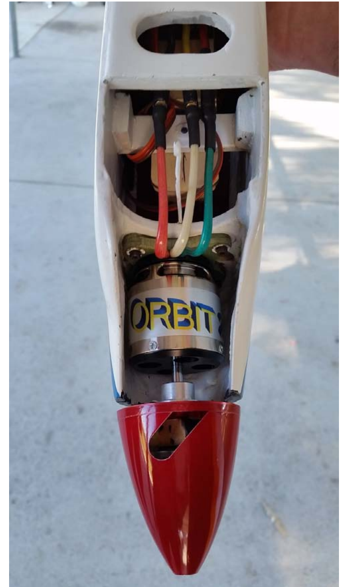
The power end of Joe Parisi's electric stunt model - Plettenberg Orbit outrunner.
