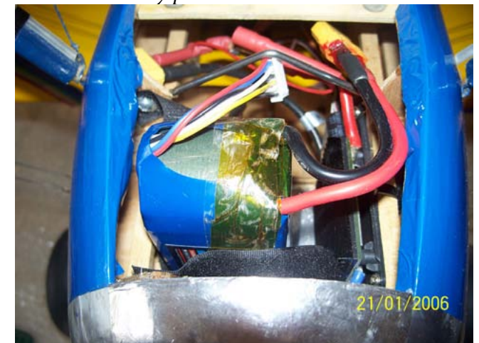
Below - battery placement with Rx batteries too!
