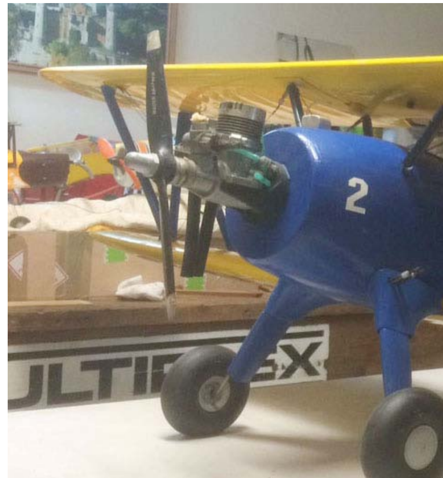
The Stearman in its original form with a huge glow motor. Ian Swadling removed the motor and all its accoutrements. In went a large Scorpion motor and all the electric bits. See the front page for the new, electric version. See the next page for some of the modifications.
