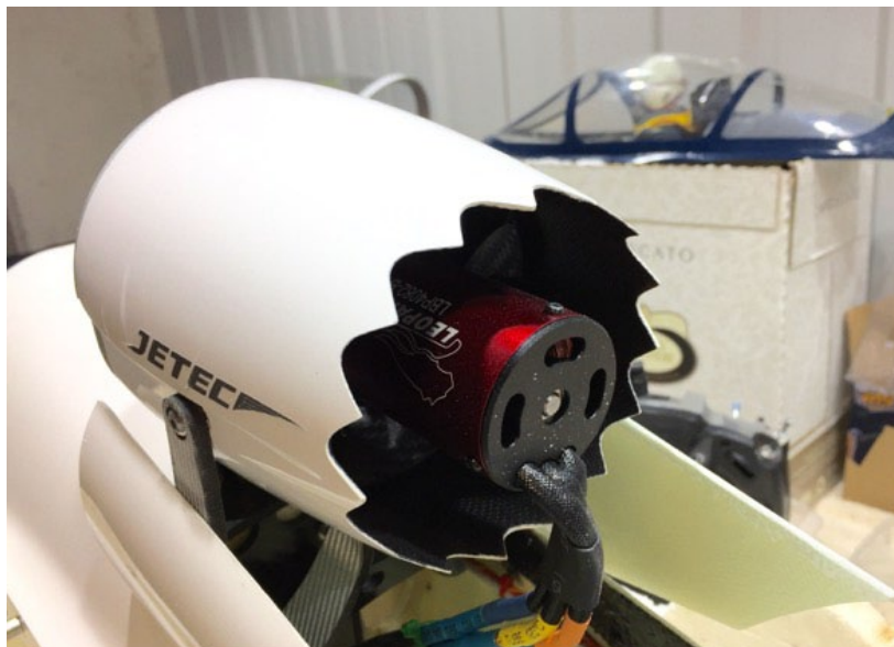
Retractable ducted fan unit in Byam's Ventus
