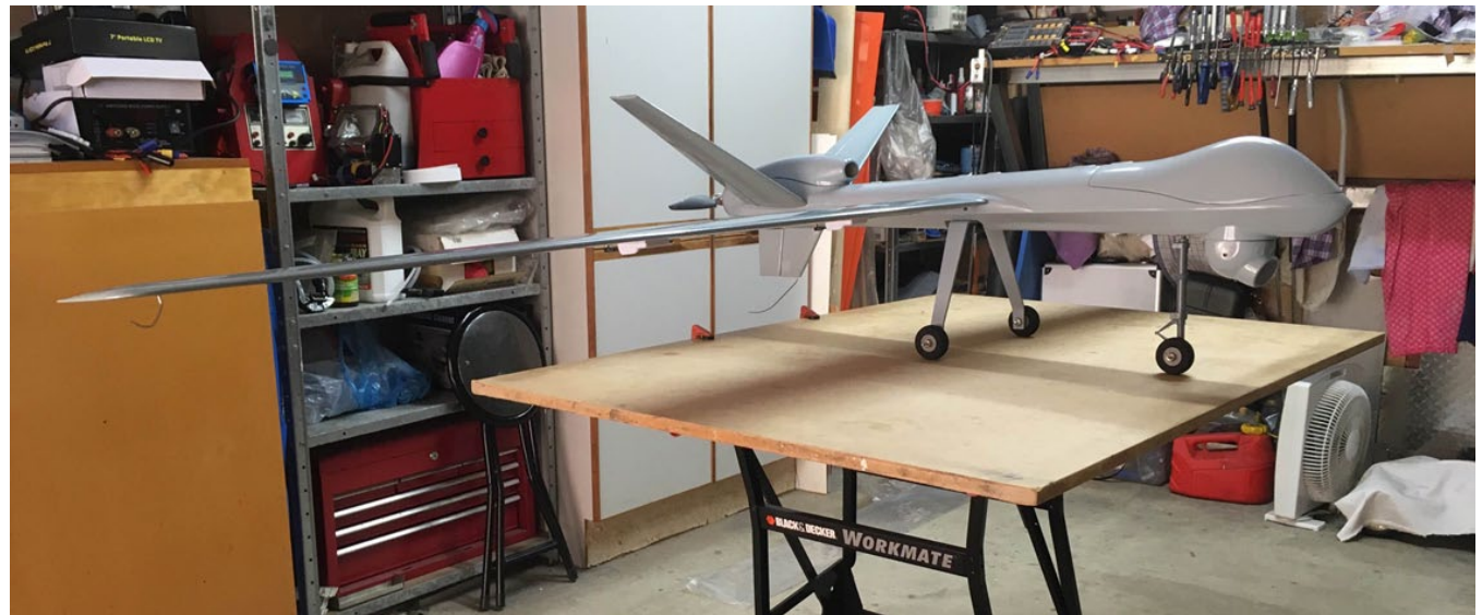
Predator surveillance aircraft by John Smith of Kingscliff - fully moulded model with pusher motor and V-tail.
