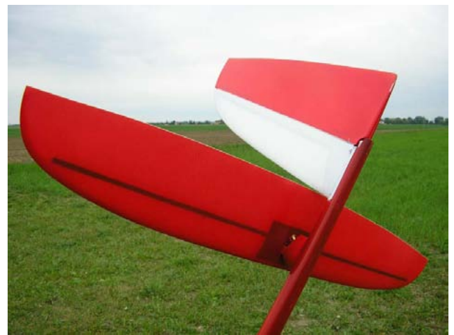
Stork tail group - devoid of protrusions that cause drag
