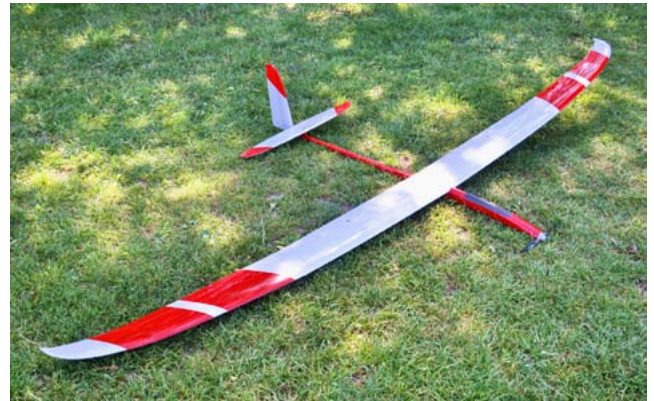
Stork fully moulded F5J machine from Slovakia - light weight, thin fuselage, 27mm diameter geared outrunner motor and 850-3S LiPo
