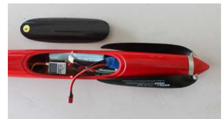
Note thin nose on the Pulsar - typical of new breed F5J machines - and how all the gear is stored well forward - aids balance, contributes to low weight.
