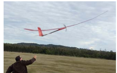
First launch by Terry - plenty of power from an MVVS 4.6/840 motor - outrunner in a case.
