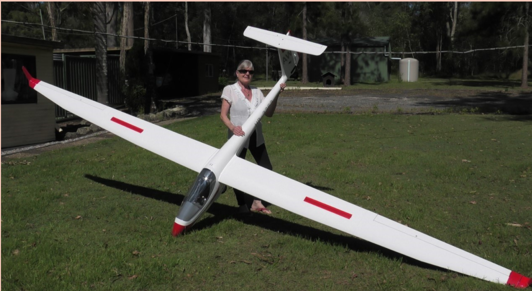
ASW28 by Claus Grimm. 5.5m wing-span, 9kg weight, Scorpion 4025-520 motor on 6S swinging a 14x8" prop. That's Mrs Grimm holding and they live in Jimboomba, SW of Brisbane.
